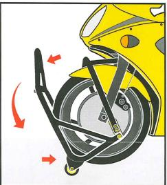
After securing the steering stem with the lift pins and the rear has been lifted, make sure all hardware are tightly secured as well. Then start pushing the handle downward while sliding the wheels forward indicated by the red arrows.
