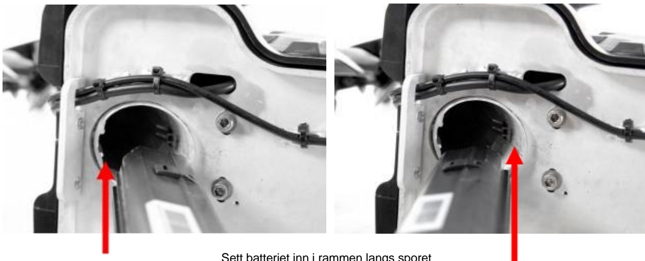
Sett batteriet inn i rammen langs sporet
